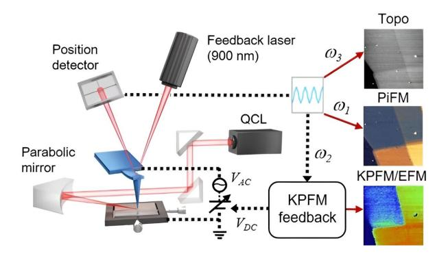
Schematic diagram of hybrid nano-microscope. Credit: Korea Research Institute of Standards and Science (KRISS)
